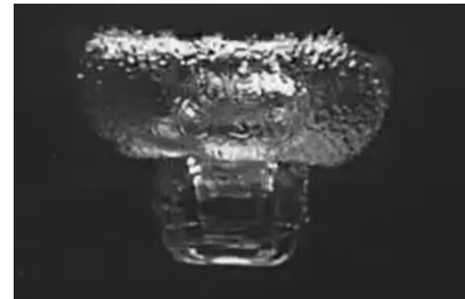
Bubble collapse with compression shock wave (Implosion)
