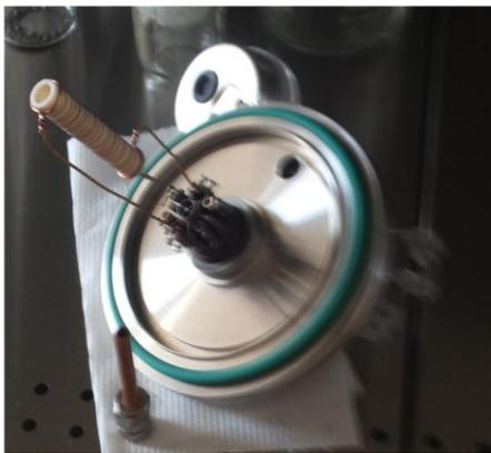
Photo 3: bottom closure with vertical heater
