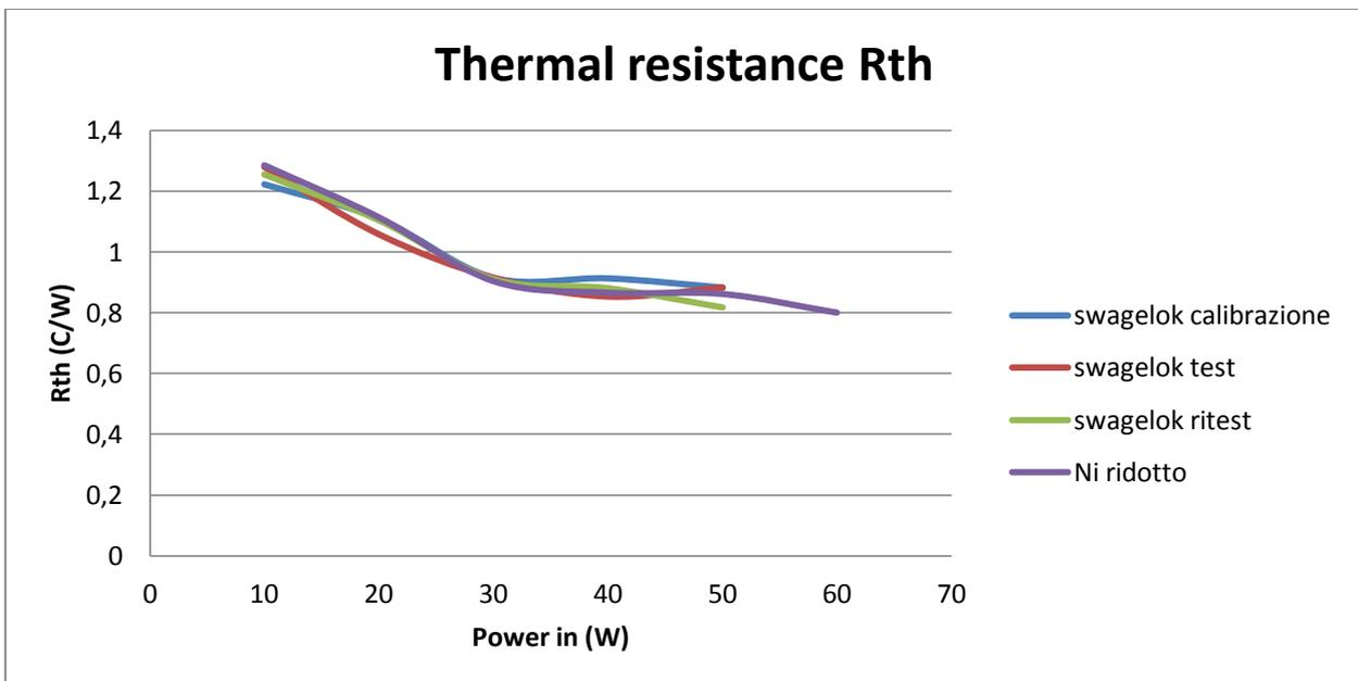
Graph 4. The Rth behavior does not show any anomaly inside the reactor.
