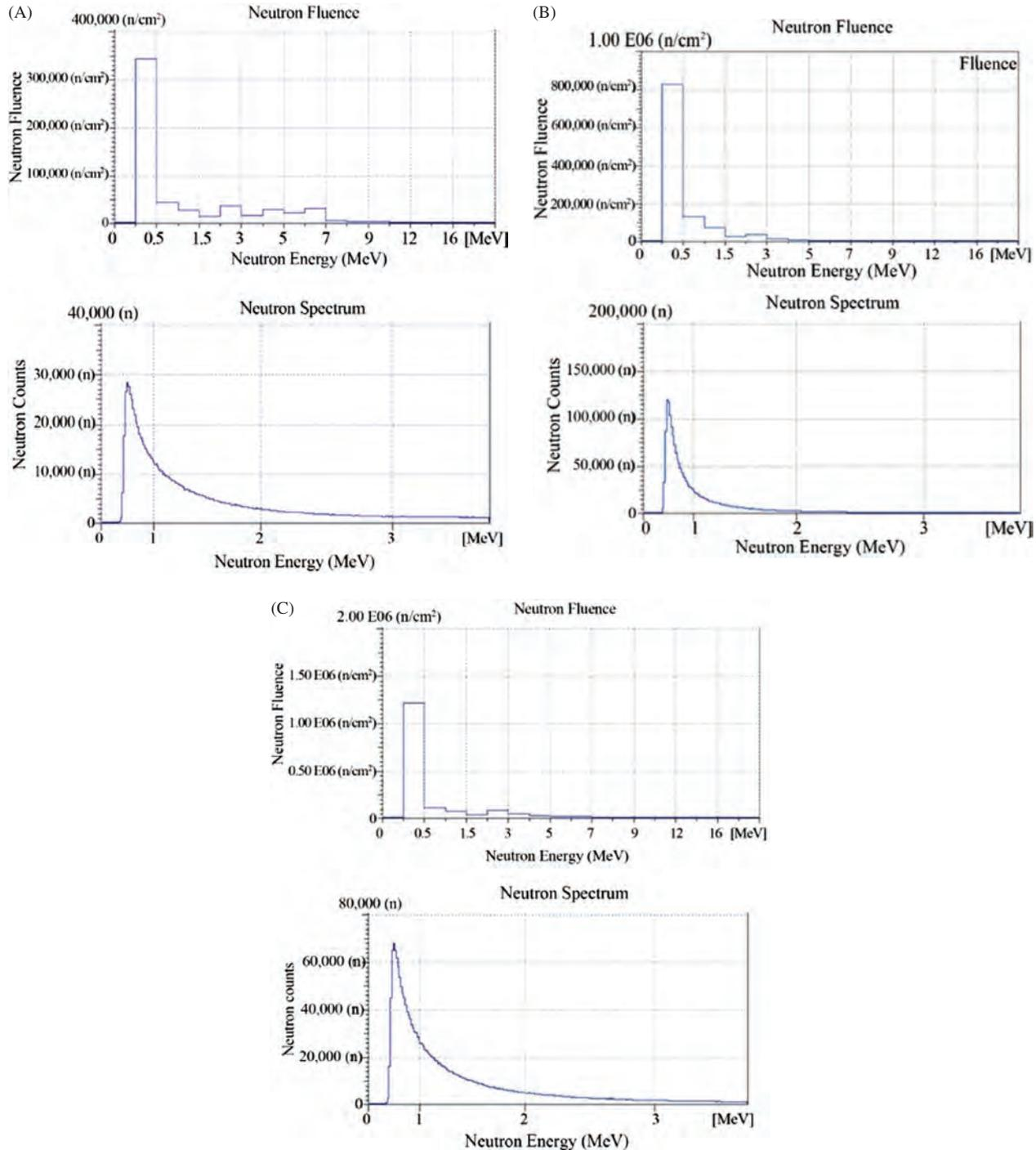
**Fig. 6.** (A) Fluence and neutron spectrum of the source TRIGA thermal column horizontal channel (long slid diaphragm). (B) Fluence and neutron spectrum of the source TAPIRO radial channel 2 (circular diaphragm). (C) Fluence and neutron spectrum of the Am-241-Be source (without any diaphragm).
