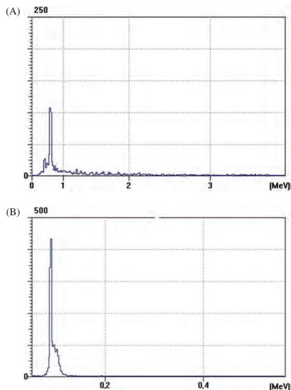
**Fig. 3.** Deformed space time (DST) neutron spectrum in details: (A) 0.3–3 MeV, NaI(Tl) liquid scintillator detector, (B) 0–0.3 MeV, Helium-3 gas detector.
