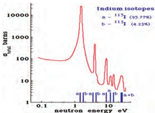
**Fig. 9.** Indium neutron activation cross section.
