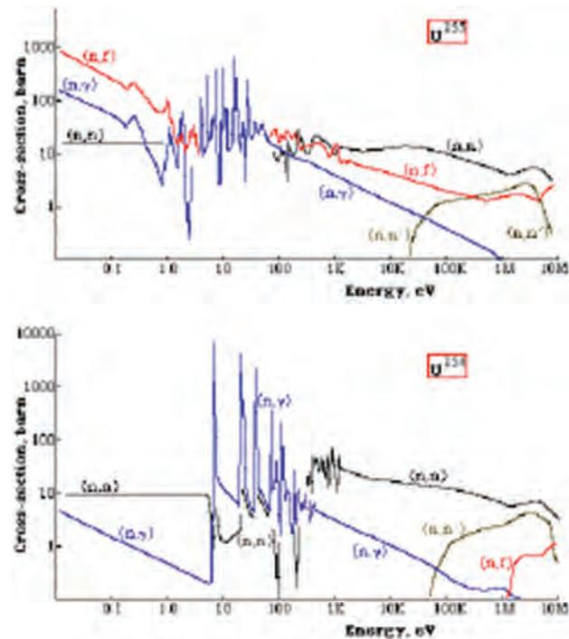
**Fig. 10.** U-235 and U-238 neutron cross sections.
