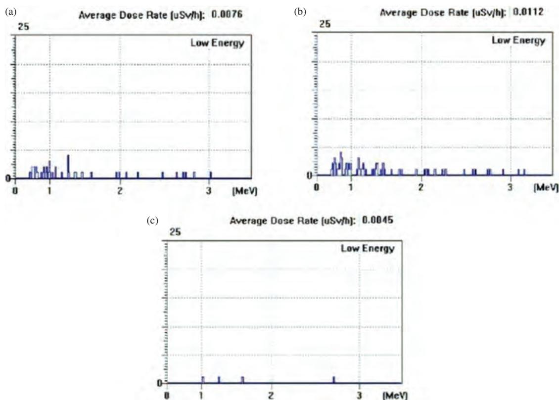
**Fig. 1.** Left, neutron spectrum from the bar of ferrite; right, neutron spectrum from the bar of steel; bottom, neutron spectrum of the background. For all of them we have MeV on the abscissa, counts on the ordinate.
