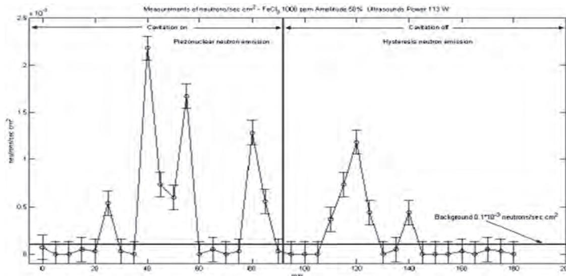
Fig. 4. Time asymmetry of neutron bursts from DST emissions.
