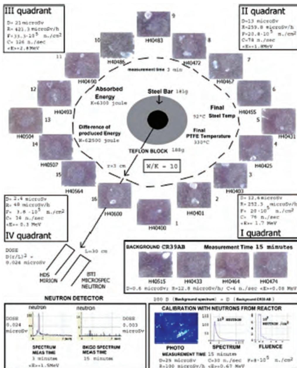
**Fig. 8.** R-0-L/S reactor horizontal view, showing the AISI 304 steel bar inserted in and surrounded by PTFE cylinder, and synoptic summary of measurements. Externally, by moving anticlockwise from n.1 to n.16, the icons of the CR39 AB detectors with the traces of the alpha particles generated by the neutron impact.
