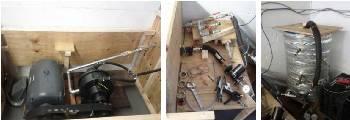
Figure 5: Cavitation heat pump setup to Increase efficiency, solid pipe connections and insulated tank
