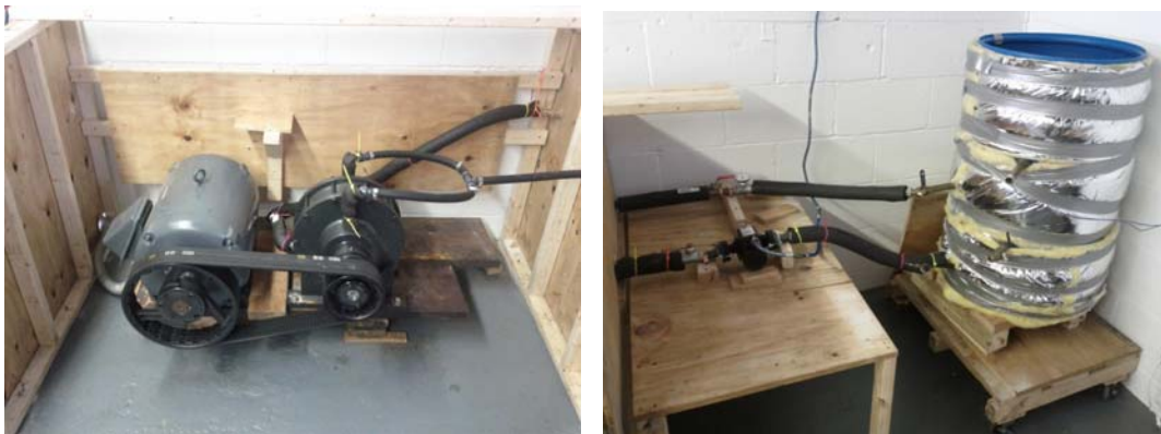
Figure 3: Cavitation heat pump setup to Increase efficiency and insulated tank
