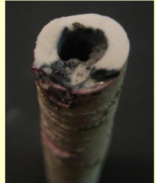
The main problem: short lifetime operation of the reactors, connected to the destruction caused by local overheating.
