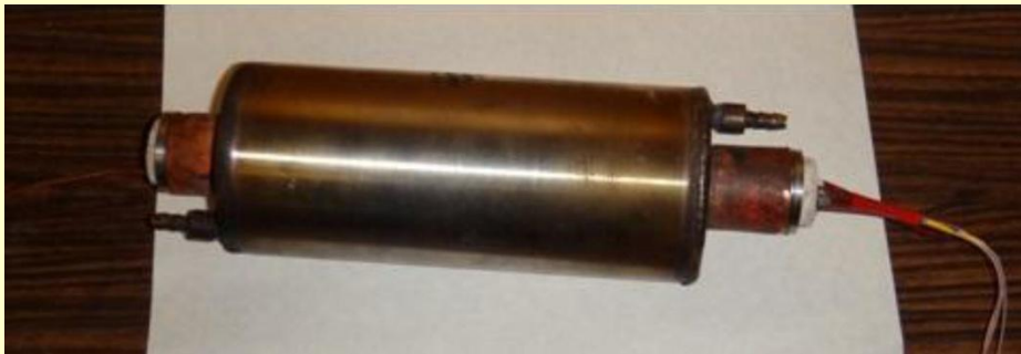
Flow calorimeter cell without the outer thermal insulation
