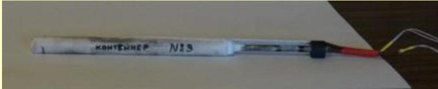
Ceramic tube with fuel and thermocouples sealed with temperature-resistant cement.
