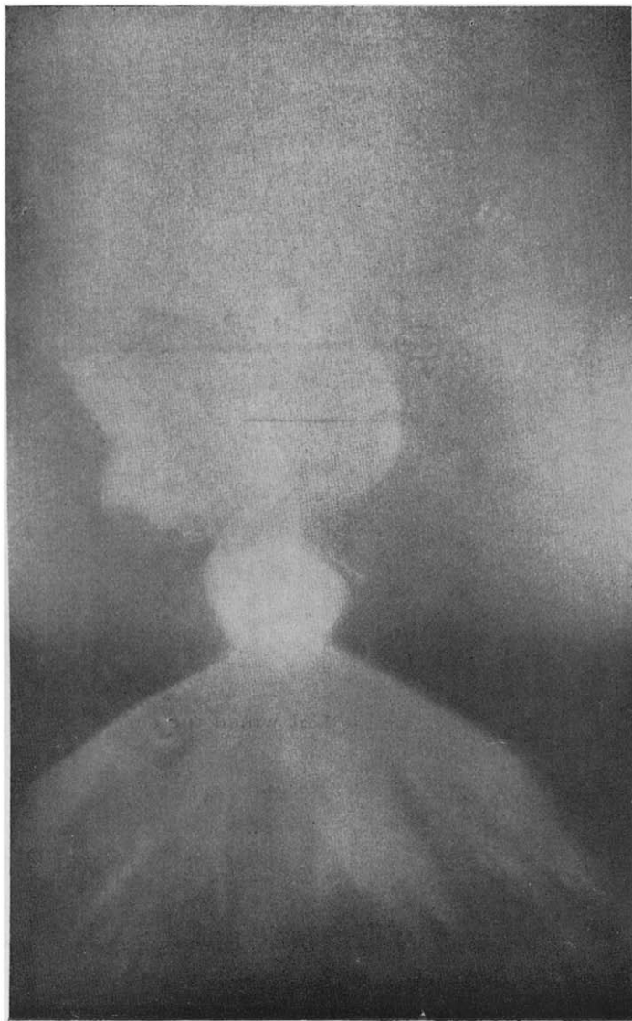
FIG. 5.—Photographic sweep of a discharge in deuterium at a pressure of P_0 = 10 mm Hg. Hemispherical electrodes were held 45 mm apart in a 180 mm diameter chamber. I_{\max} = 1.2 \times 10^6 amps, T/4 = 9.5 \mu\text{sec} . Scale: 18 mm = 1 \mu\text{sec} .
