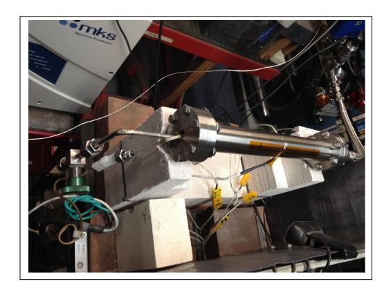
A type K thermocouple is mounted near the center of the cell, with two wraps of 30 gauge Nickel wire to secure it and some Kapton tape for electric insulation. A small dab of white heat sink compound is applied under the junction to improve the thermal coupling with the cell tube.
