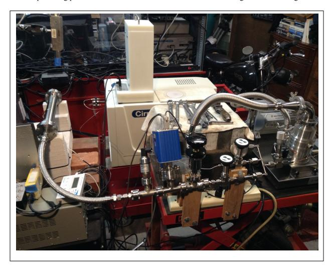
The new cell is 1.5" OD SS304 tubing with Conflat 2.75 end caps. It was made by LDS Vacuum Systems, \$180 fully polished, cleaned and tested at 1E-5 Torr. A locally fabricated 3/8"(ID) x 10" x .062 SS304 thermo-well is TIG welded into one end cap. A small VCR tube and valve for mass spec. gas sampling was also added. The DC-powered 300 watt 5/16 x 5" cartridge heater is inserted into the thermo-well tube.
