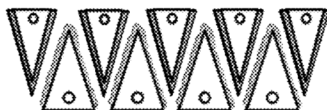
Figure 33: Alternate arrangement of working and counter electrodes
