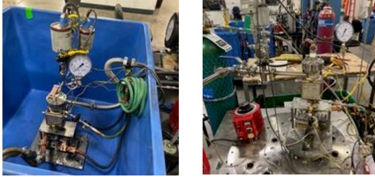
Figure 1. Photographs showing two separate molten metal cells that also served as molten metal calorimeters. Cells A (left) and B (right) were used for validation and will be referenced in this report.
