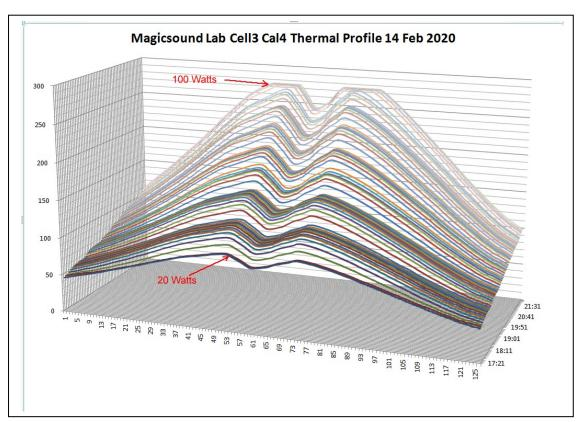
Here's a rendering of the cell thermal profile during the entire 5 hour calibration. The data is generated by the Optris camera PIX software, with 125 points along the cell axis sampled every 5 minutes.
