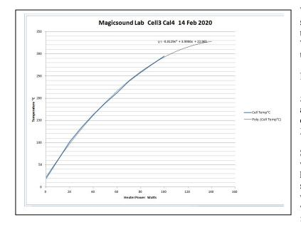
The temperature shown is the hottest spot, at the center of the cell tube where the two thermocouples are mounted. Tracking is very good, within  $\pm 1^{\circ}$ C over the entire range.
