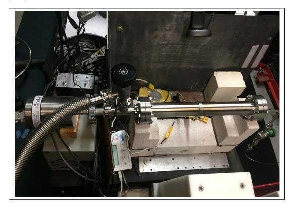
Initial calibration showed that mounting the thermocouple with Kapton tape and thin wire was not stable over time. It was replaced with two calibrated Omega type K probes, secured with a hose clamp. This is very secure and solid, with good data yielded by the next calibration (with 1030 Pa of H2 in the cell):
