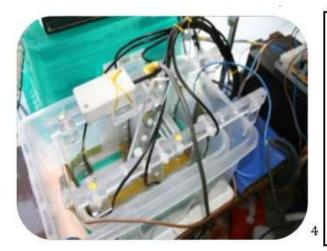
Here you can see a set-up typical of those used to grab data while electrolysing catalytic carbon. There are six thermossensor pairs which are submerged close to the anode and cathode (not seen here) with the third pair central in the tank. The infra-red sensor sits above the liquid surface. In the RHS can be seen the Geiger counter tube which (not shown here) was submerged in the tank for some runs.
