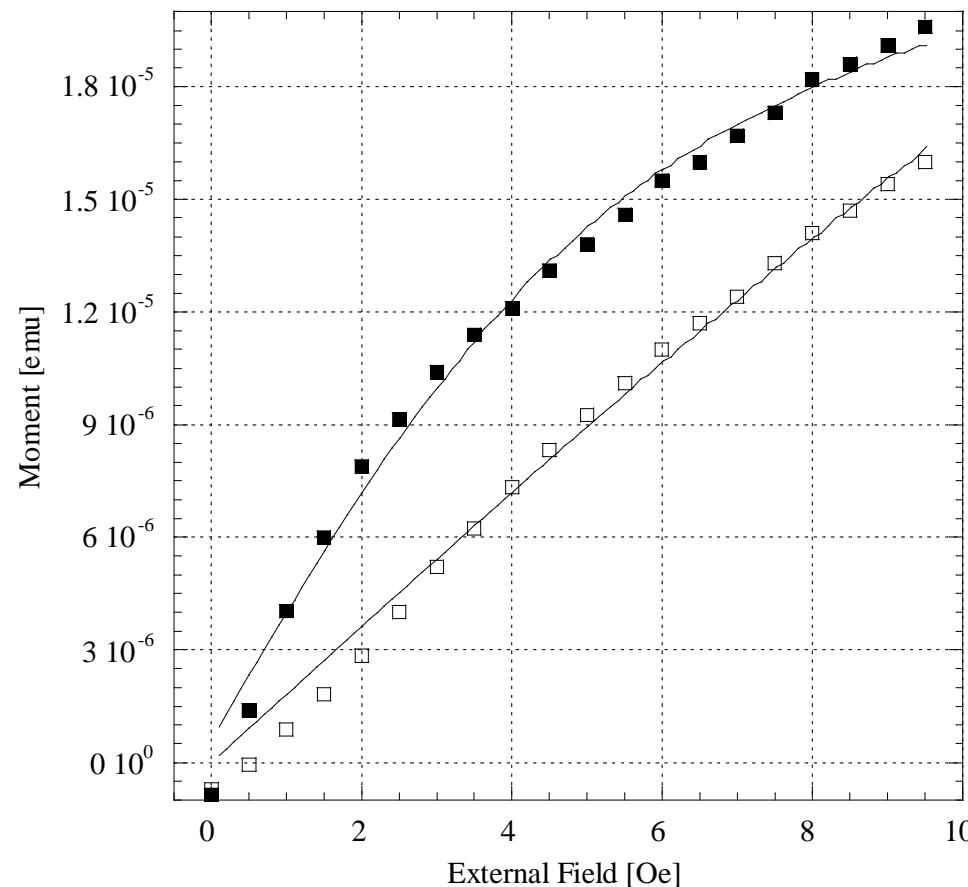
Net magnetic moment (PdHx-Pd) versus external field at 2 K. The strong diamagnetic response at low field (<50e) and irreversible behavior are characteristic of a type II superconductor with magnetic flux pinning.
