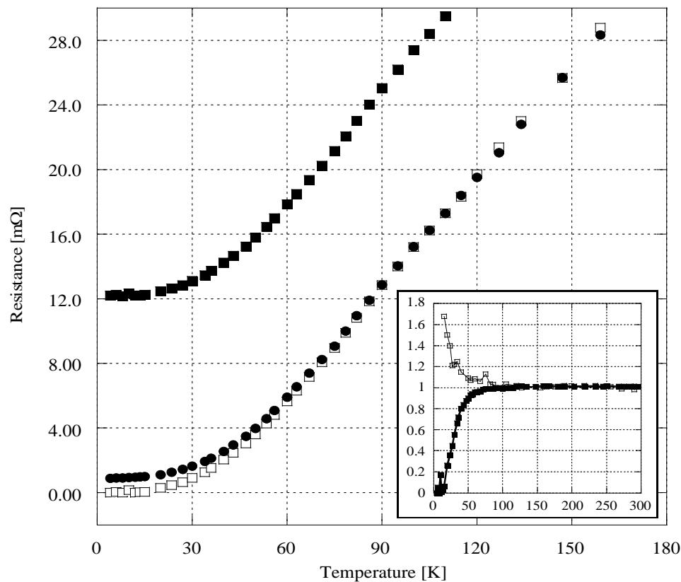
Normalized V-I characteristics for (Pd/PdOHx)/(Pd/PdO) ratio vs.T. Resistance decrease with decrease in I below 60 K.
