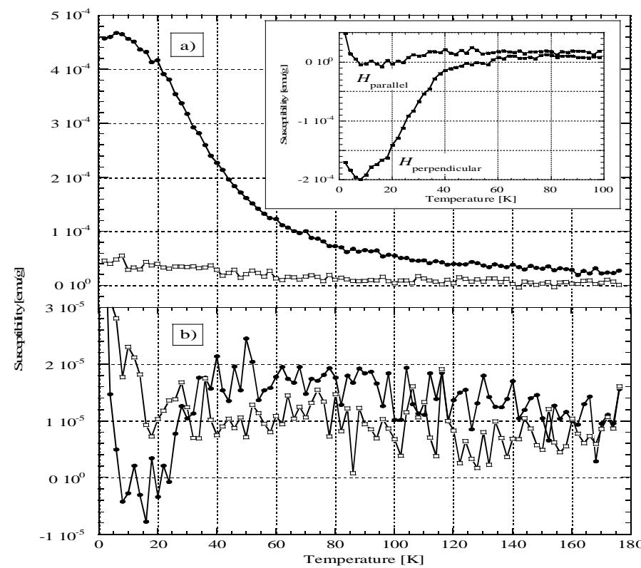
X' AC susceptibility of Pd/PdO:Hx and Pd/PdO-blank samples vs. T for  $H_{\perp}$  and  $H_{\parallel}$  with respect to the sample:  $H_{\perp} / H_{\parallel} = \xi^2/d^2 = 25$  at T=10 K; d ~ 50 nm (Pd-PdO interface width),  $\xi \sim 250$  nm – 2 dimensional type II Superconductivity
