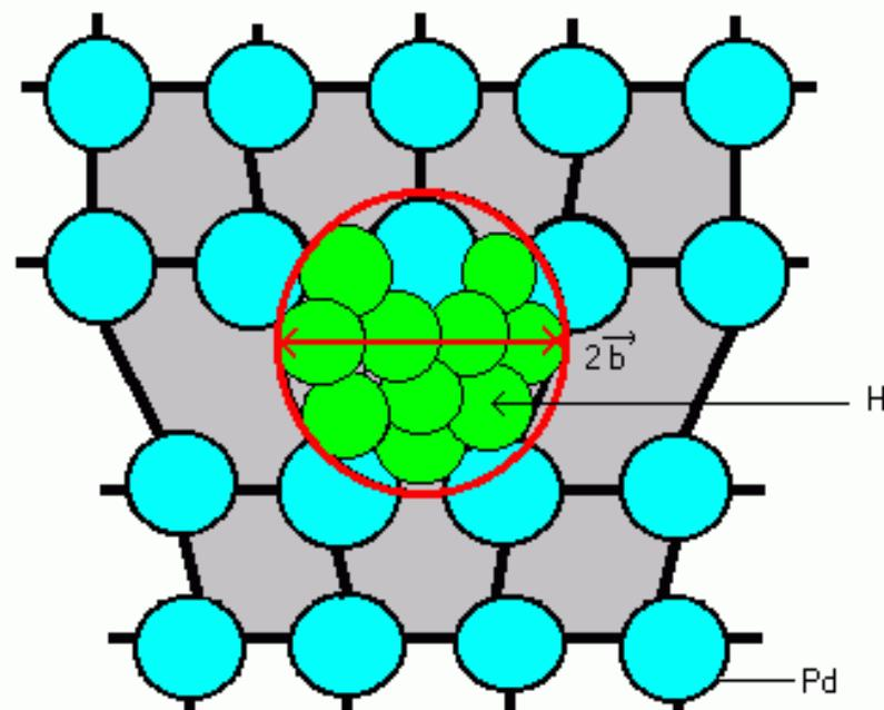
$$\begin{array}{l} \text{Pd}(1\bar{2}\bar{1}) \\ \rightarrow \\ b[\bar{1}01] = 2.75 \text{\AA} \end{array}$$
