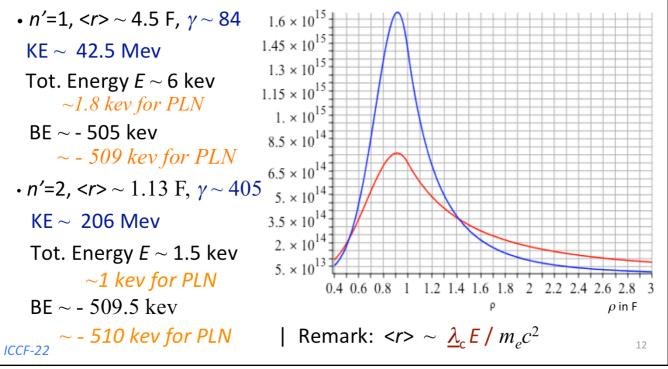
Here we plotted the curves of probability density corresponding to values 1 and 2 of radial number.
