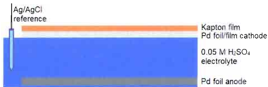
Figure 10. Side view of aqueous electrochemical cell. A 25\ \mu\text{m} Pd foil or 50\ \text{nm} Pd thin film is attached to a 127\ \mu\text{m} X-ray transparent Kapton film. A 25\ \mu\text{m} Pd foil is used as anode. An Ag/AgCl reference electrode is inserted into the cell to provide a potential reference. The entire cell is filled with 0.05\ \text{M}\ \text{H}_2\text{SO}_4 electrolyte. An image of the actual cell can be found in Figure 6.
