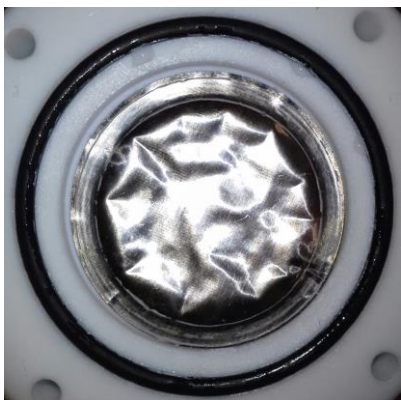
Figure 4. The Pd cathode after few hours of operation in the cell
