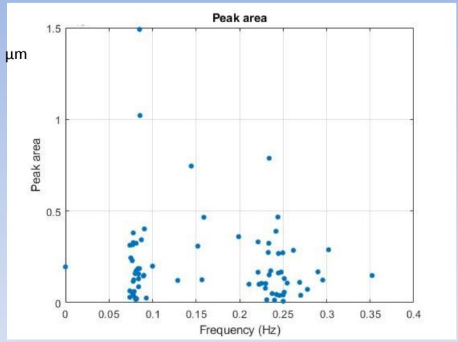
1  $\mu m$  displacement equivalent to 1.3  $\mu N$  Resonant thrust 0.04  $\mu N/W$
