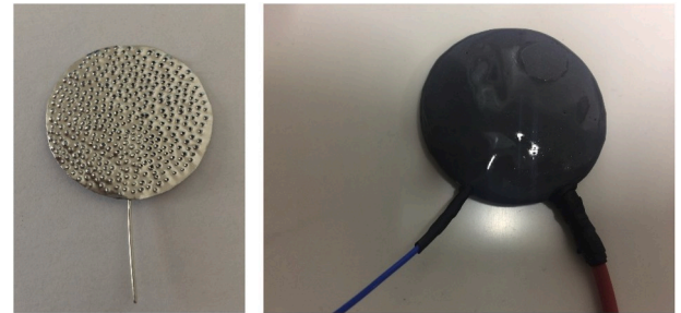
Fig. 11. Leakage current capacitor with perforated cathode.
