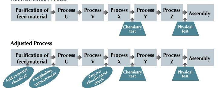
To fabricate new Fogbank, modern scientists reconstructed the historical manufacturing process (*top*). However, when the resultant Fogbank assembly did not meet quality requirements, scientists analyzed the historical manufacturing process and discovered one minor difference that, when adjusted properly (*bottom*), yielded quality Fogbank.
