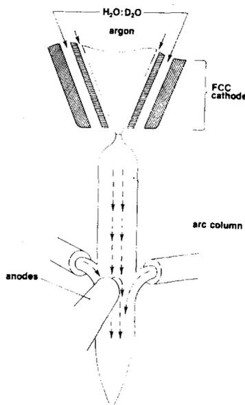
FIG. 1. Scheme of dc arc with fluid-convection cathode and three anodes.
