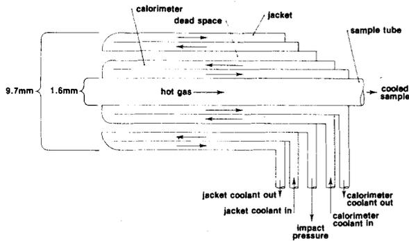
FIG. 2. Scheme of Calprobe nozzle.
