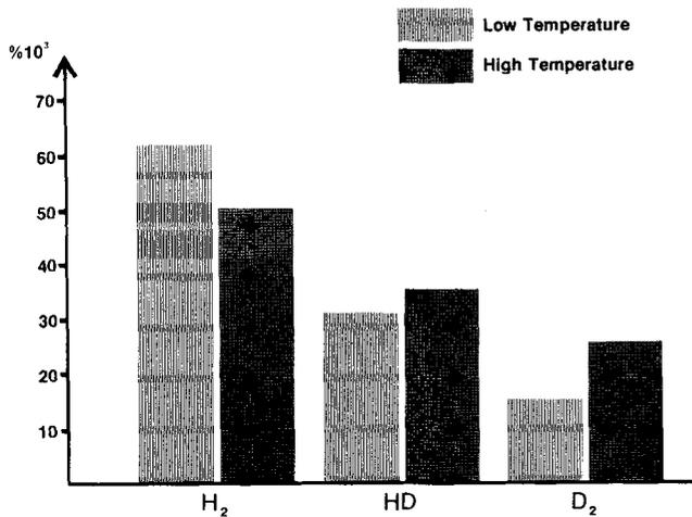
FIG. 3. Mean values of volume percentage for D<sub>2</sub>, HD, and H<sub>2</sub> for samples taken at high- and low-temperature regions.
