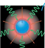
X-rays vaporize outer layer of fuel pellet, which bursts outward and imparts inward momentum to the hydrogen fuel.
