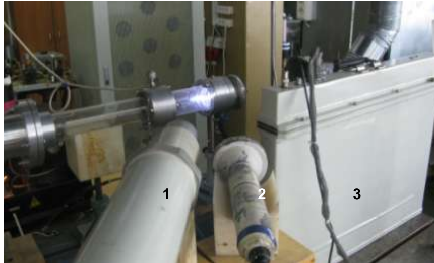
Figure. 2b. General view of the experimental set up PVR with detector SPRS (1- \gamma -detector, 3- neutron detector) and neutron radiometer KRAN-1 (2)
