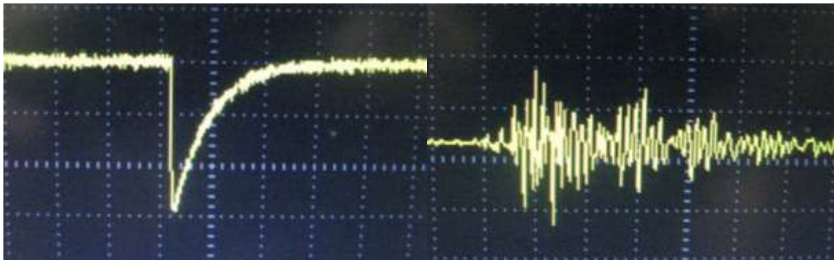
Figure 9. The typical neutron's signal (left) from the calibrator Na22 (20 \mu s/div) and typical neutron-like signal (right) from the HP (50ns/ div) recorded by radiometer KRAN-1.
