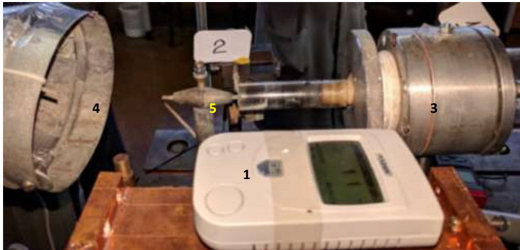
Figure.7. RF-films with thin Al -filters (2) and Geiger's counter (1) near PVR' nozzle (3). Gas flow ejector- 4, thermocouple- 5
