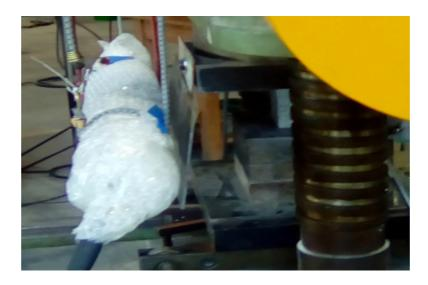
Figure 5: The mechanical press, the granite block inside its jaws and the detector, suspended and wrapped in a white protective plastics. The <sup>3</sup>He detection system was recalibrated against thermal neutrons with this protection in place.
