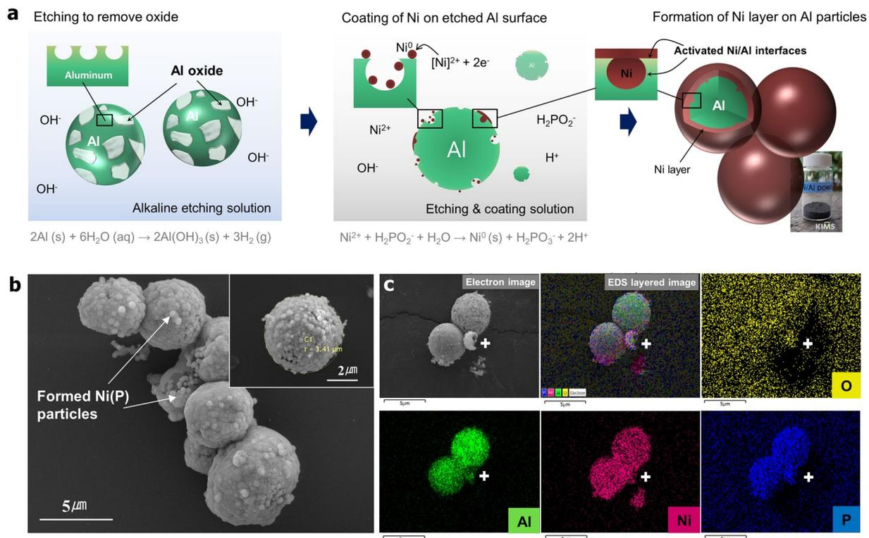
**Figure 1.** (a) Schematic illustration of removal of surface oxide by NaOH etching solution, forming a Ni layer on Al particles with nanosized craters dispersed on their surfaces. (b) Surface morphology of the synthesized Ni/Al particles. (c) EDS maps showing O, Al, Ni, and P distributions.
