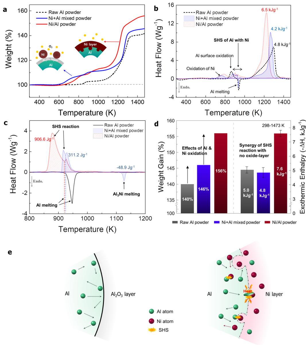
**Figure 3.** (a) TGA and (b) DSC results with increasing temperature in air atmosphere (heating rate of 10 K min<sup>-1</sup>), (c) changes in heat flow as a function of temperature in Ar atmosphere (heating rate of 10 K min<sup>-1</sup>), (d) comparison of weight gain and exothermic enthalpy energy of fine Al particles, mixed powder, and Ni/Al powder, (e) schematic illustration of SHS reaction in activated Ni/Al interface compared to that in surface-passivated Al.
