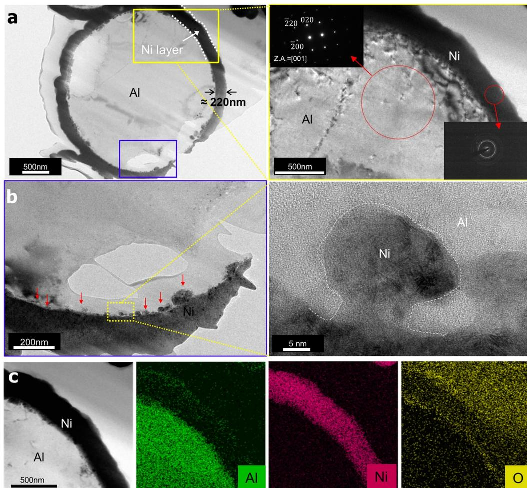
**Figure 2.** (a) Cross-sectional TEM image of Ni/Al particle and enlarged microstructure of zone indicated by the yellow box. (b) Enlarged TEM image of the zone indicated by the blue box in (a) to show the rough Ni/Al interface and nanosized crater filled by Ni material. (c) EDS maps of Ni/Al particles showing the distributions of Al, O, and Ni atoms.
