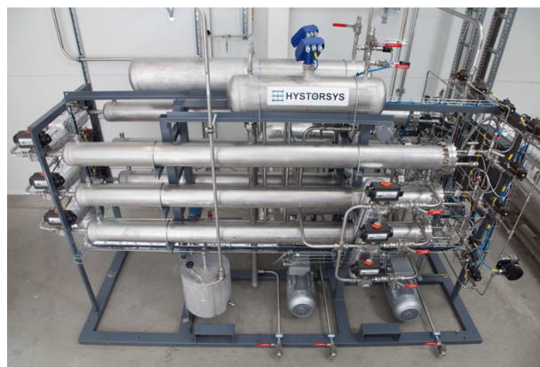
Fig. 15 HYMEHC-10 proof-of-concept compressor at HyNor Lillestrøm
