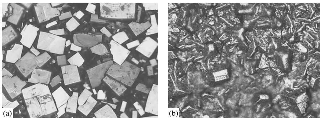
**Fig. 3.** Optical microphotographs of the surface of the polycrystalline diamond film before (a) and after (b) irradiation of the target by a deuterium-ion beam. The image dimensions are  $500 \times 370 \mu\text{m}$ .
