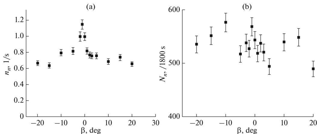
**Fig. 6.** Dependence of the count of the neutron detector on the angle of rotation of the diamond target in two cases: (a) the detector based on  $^3\text{He}$  counters (the target is oriented towards the neutron source by its growth side); (b) the scintillation detector operating for a time of 1800 s (the target is oriented towards the neutron source by its growth side; the threshold of recording recoil protons is 150 keV in the electron equivalent).
