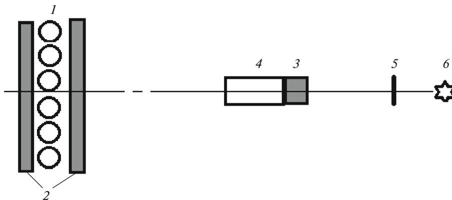
**Fig. 5.** Scheme of arrangement of the  $^{252}\text{Cf}$  neutron source, detectors, and the target in the second series of measurements: 1—detector based on  $^3\text{He}$  counters; 2—organic glass; 3—scintillator (paraterphenyl); 4—photomultiplier tube; 5—diamond target; 6— $^{252}\text{Cf}$  neutron source.
