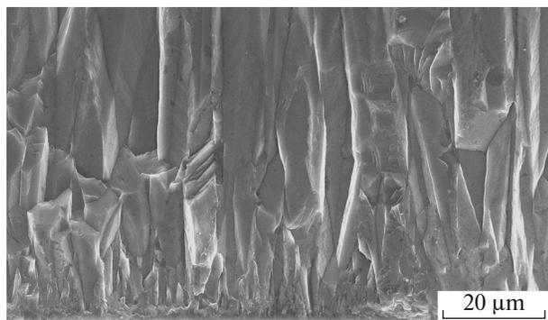
**Fig. 2.** Image of a polycrystalline diamond film in the transverse section obtained by using a scanning electron microscope.
