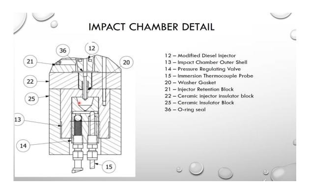
During the collision enormous hydraulic pressures collapse the bubbles within the injection volume. Cavitation bubbles have the remarkable ability to focus intense energy and forces during their collapse. The resulting heat energy contributes to the continuous creation of superheated steam inside the impact and expansion chambers, creating a Plasma where before there was water vapor.
