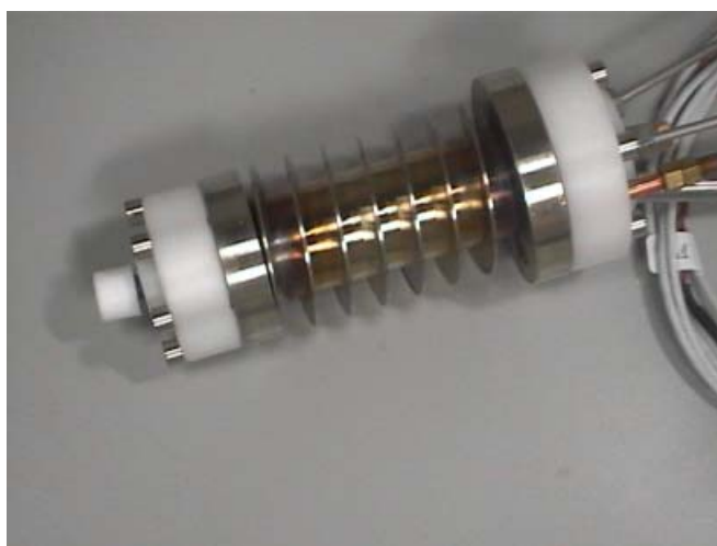
Figure 3 A view of the glow-discharge cell. The channels between the spiraling fins are for coolant flow
