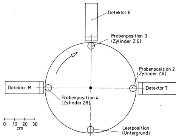
**Fig. 14:** schematic drawing of the ECS5 experimental arrangement using three detectors R, E, T and three electrolytic cells with cathodes Z5, Z6 and Z8 located in a water bath, that can be turned around
