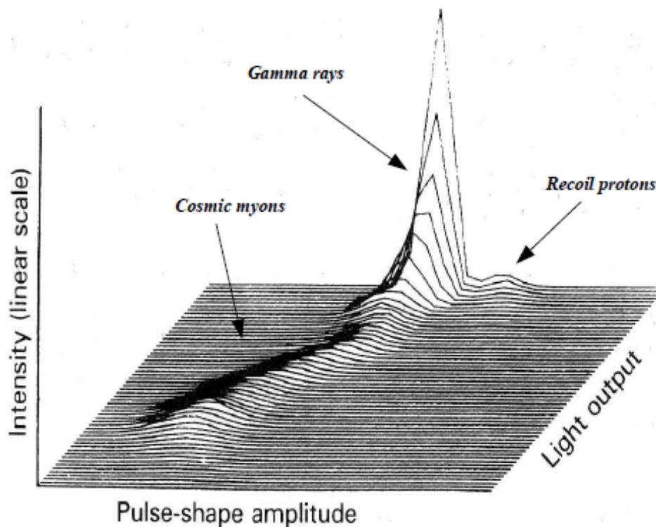
*Fig. 2: Three dimensional background spectrum versus light output and pulse-shape signal amplitude for the recoil proton spectrometer used. Very few fast neutrons are contained in the background spectrum only.*
