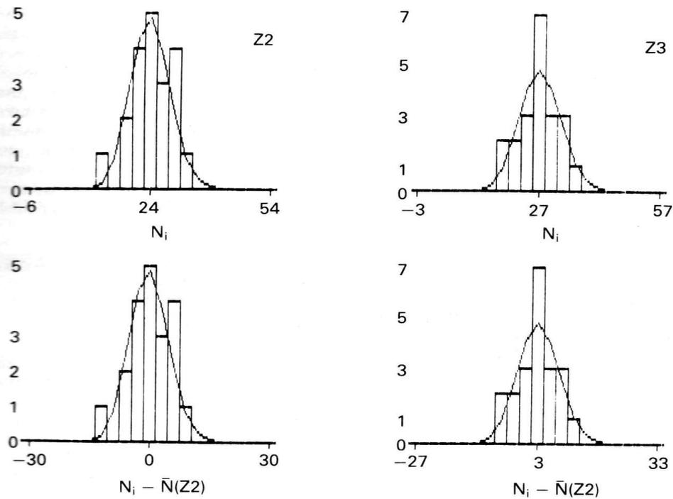
**Fig. 3: Distributions of 1h counting rates  $N_i$  in recoil energy group 1,9...2,9 MeV for palladium probe Z2 (without electrolytic current) and Z3 (with Deuterium loading) within the time interval from 100h to 200h of electrolysis (upper part) and relative to an averaged background line obtained from the Z2-measurement (bottom). The Z3 measurement shows an average effect count of  $3 \text{ h}^{-1}$  over 100 hours comparing to Z2 probe. Smooth lines represent Poisson distributions.**
