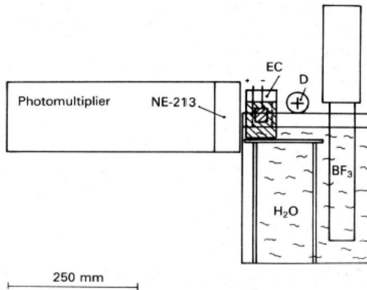
*Fig. 1 Schematic of experimental arrangement: EC – electrolysis Cell; H<sub>2</sub>O – water basin; D – position of various other detectors; the heavy iron shield is not shown*
