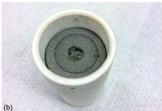
Figure 65.—Test disk stack placed within the reactor. (a) Ceramic holder with test disks in reactor. (b) Test disks in ceramic holder. (c) Test chamber.
