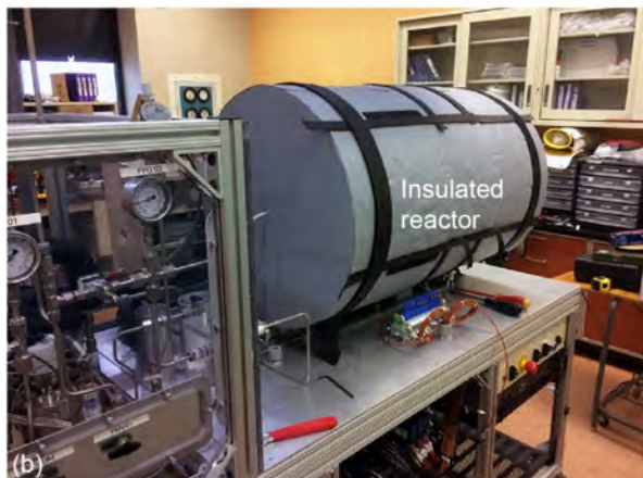
Figure 8.—Plasma reactor test stand. (a) Test stand side view. (b) Insulated reactor. (c) Test stand.
