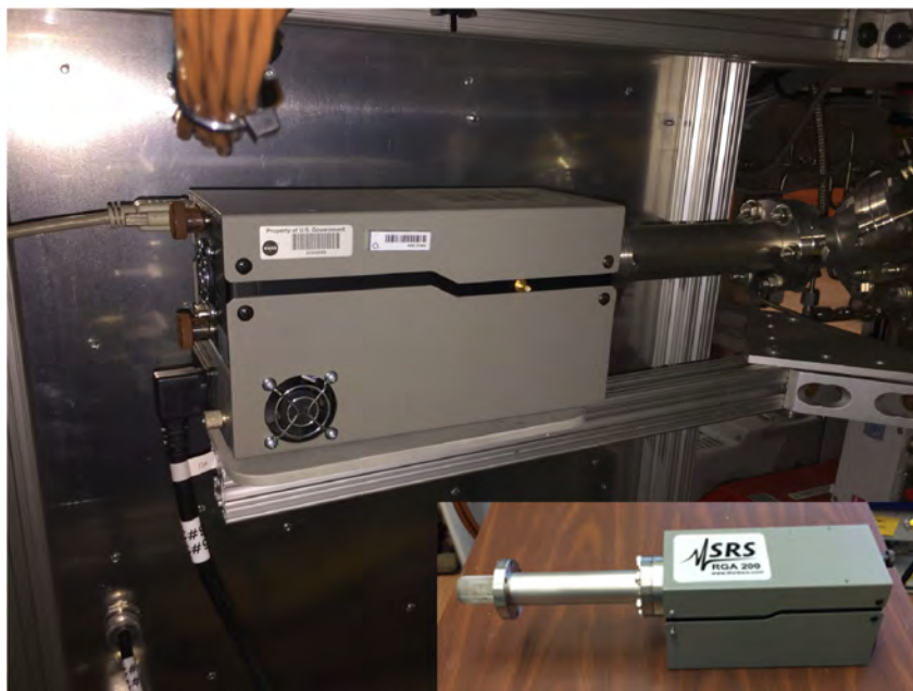
Figure 60.—Stanford Research Systems (SRS) residual gas analyzer (RGA) model RGA200 installed in test stand. Inset shows uninstalled SRS RGA.
