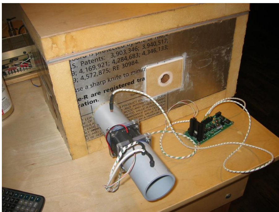
Figure 2: Calorimeter Enclosure showing fan, temp sensors on inlet port
