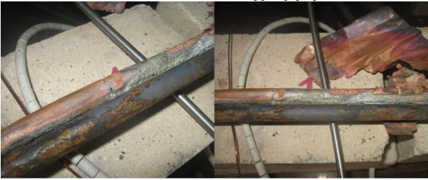
Steam began to escape between the bricks and... (the next part is not clear exactly)... the gaps (?) did not reach the cooling vessel. The silver-soldered connections melted (Editor's note: 750C approx) and holes appeared in the copper pipe.
