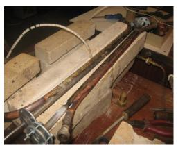
Next we connected a 4-way hydraulic system. This allows for direct flow of cooling water through two reactors in series, parallel or individually.
