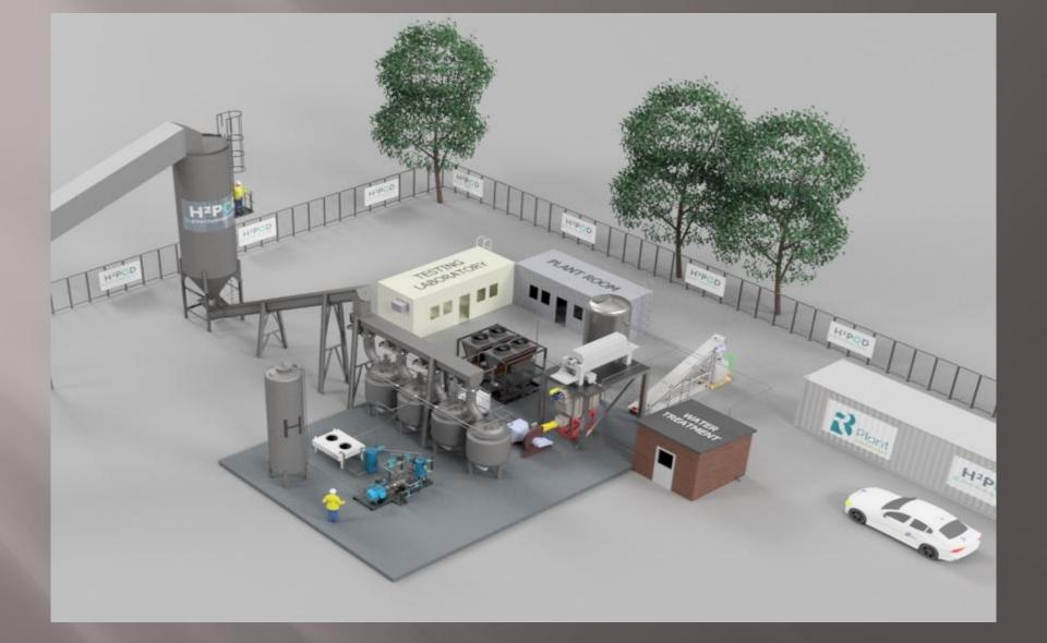
Plant design (by RB Plant Ltd) to produce 150 t/y H2 and over 4,300t/y ATH from 1500 tonnes of Al scrap.
