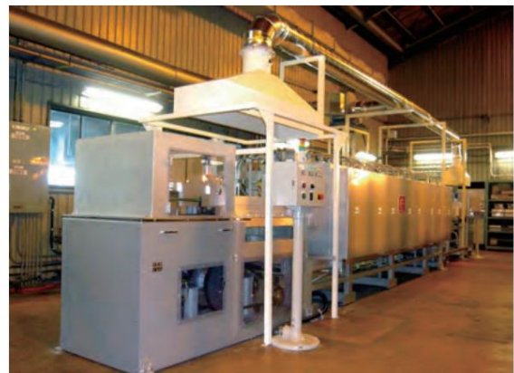
Heat treatment furnace that can reproduce the actual finish reduction conditions
