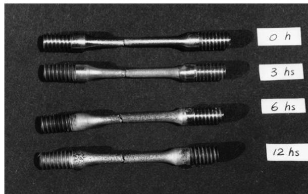
Fig. 4. The ruptured tensile specimens of 304 stainless steel with different hydrogen charging time.
