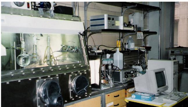
Fig. 2. The radioactive-proof electrochemical apparatus for tritium charging.
