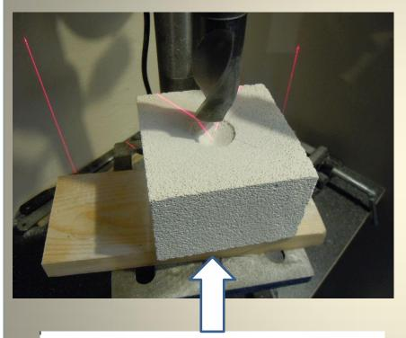
The bricks are cut into two halves and each half bored to accept the quartz tube liner and coil unit.
