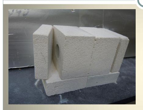
The furnace body is completed by cutting 4x 35mm thick slices from half-bricks, two for the base, one for the removable door and one for the fixed back panel.
