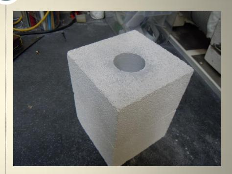
The two bored halves are cemented together using a mix of waterglass zinc oxide and magnesium oxide.
