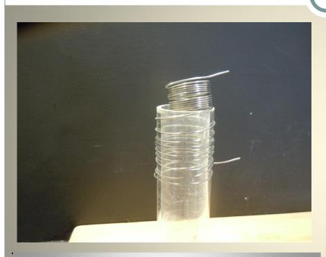
The 25mm. coil is coaxed onto a 40 x150mm quartz tube. The diameter difference ensures the heater coil is In good thermal contact with the quartz along its whole length
