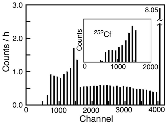
Fig. 2. Pulse height distribution of the BG counts/h accumulated for 2880 h. Inset shows that of  $^{252}\text{Cf}$  source for 3 min. The peak position is set at 1500 channel of the ADC.
