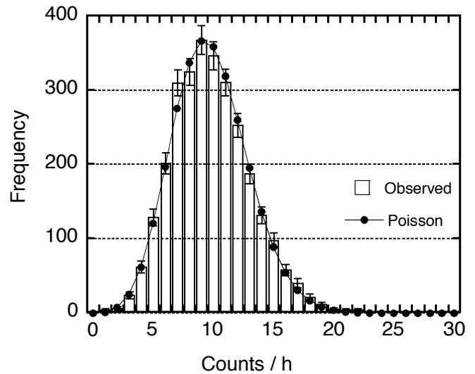
Fig. 3. Frequency distribution of the BG counts/h for 2880 h. Average is  $9.78 \pm 0.06$  counts/h. Bars are observed frequency and dots are Poisson distribution of the mean value at 9.78. From chi-squared test ( $\chi^2/\nu = 10.9/17$ ), the confidence level of the consistency is 0.861.
