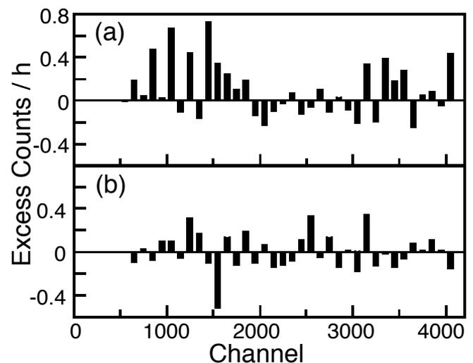
Fig. 5. Pulse height distribution of counter signals without the software cut calculated by subtracting BG signals from the counts of fracture experiments of LiNbO<sub>3</sub>: (a) the sum of pulse height distribution of the upper pressure region at 30 kPa or above, and (b) that of the lower pressure region at 18 kPa or below.
