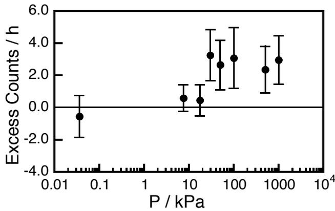
Fig. 4. Excess neutron counts/h calculated by subtracting the BG counts from the counts during the fracture process of LiNbO<sub>3</sub> from 0.036 to 1000 kPa in deuterium gas. The data at 101 kPa are taken from our previous results.<sup>5)</sup>
