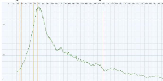
Fig.2 shows a typical noisy 10' uni directional lab background behind the experiment with an average count rate of 11.6c/s.
