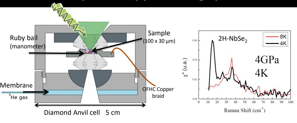
Set-up for Raman spectroscopy to probe low energy excitations (down to 5 cm<sup>-1</sup>  $\sim$  0.6 meV) under pressure (40 GPa) and at low temperature (3 K)
