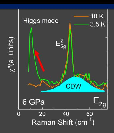
New high-pressure induced in-gap mode in 2H-TaS<sub>2</sub>
