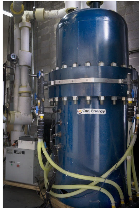
Fig 6) left: Top view of 25kW ThermoHeart® Engine. Right: photograph of engine under test.
