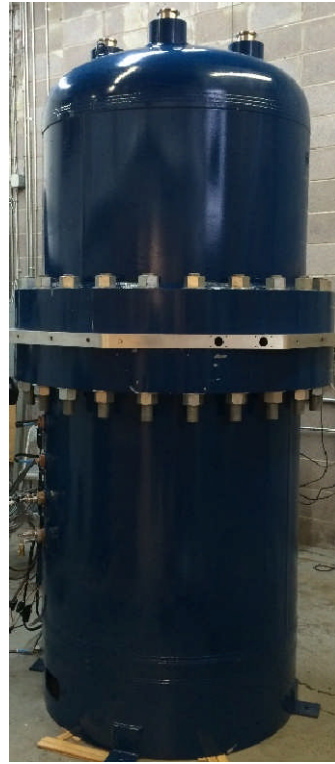
Fig 5) left: CAD of 25kW ThermoHeart® Engine. Right: photograph of engine fully assembled. The penetrations in the upper pressure vessel are the thermal heat transfer oil inlets and outlets. The heat rejection fluid is circulated through the center aluminum plate.
