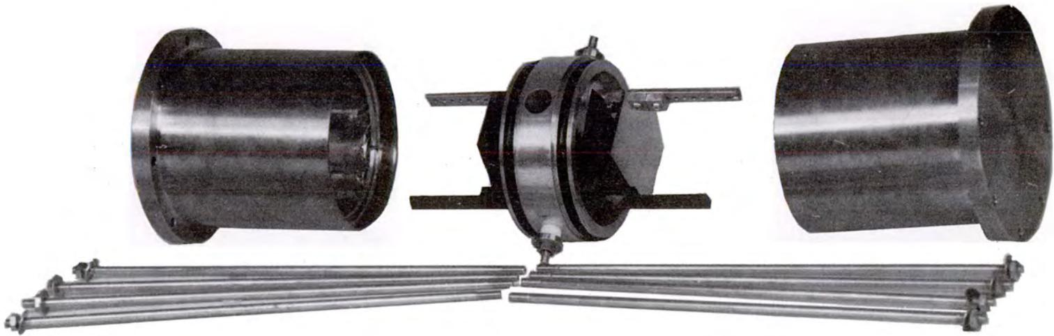
INTERLEAVED FLAT PLATE CELL, DISASSEMBLED
