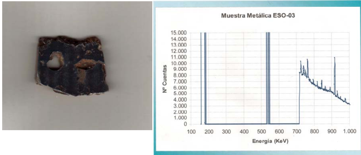
Figure 12. At left, sample ESO-03 submitted for a Prompt Gamma study at CCHEN, Santiago, Chile. At right, detail of lower end spectrum, data rechecked and certified by CCHEN and the Ministry of Mining and Energy of Chile.
