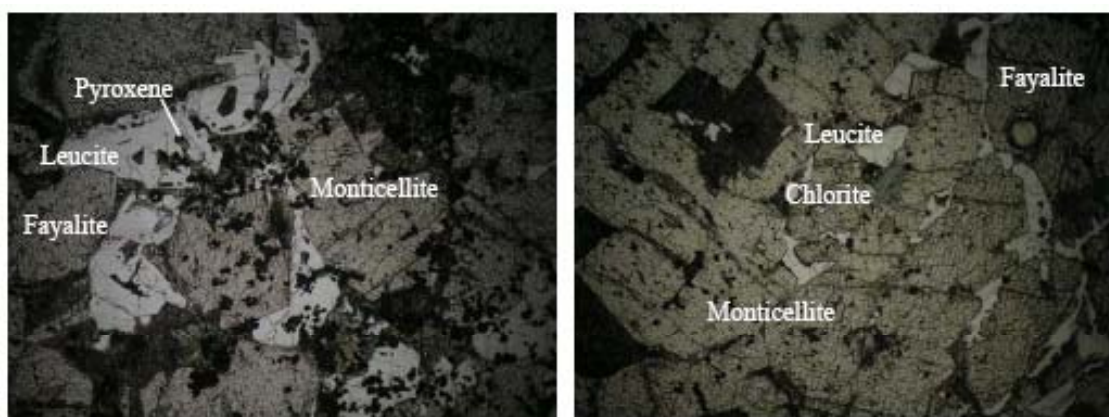
Figure 1. Micropetrographic photographs of sample Oliv01. a) Monticellite, fayalite, hedenbergitic pyroxene, leucite and opaques, among them pyrite, iron and chromium oxides, with lesser alteration chlorite. b) Monticellite, fayalite, leucite, chlorite and lesser opaques, iron and chromium oxides.
