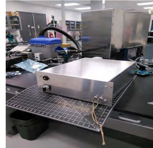
High-Current Digitally Controlled Pulser for High Current and Magnetic Field Applications
