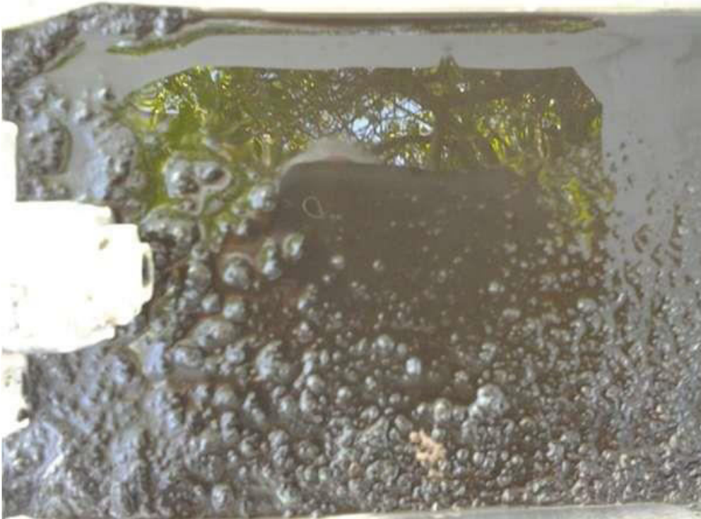
Picture# 6- after 24 hours shows all that remained of the plate.
