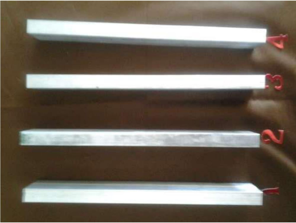
Picture #2- After 6 hours of stay in solution plates: # 2#3#4 were reduced to (8.71 x 1.1 x 0.41inches)
