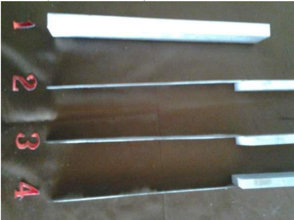
Picture# 4- After 18 hours in solution plates: # 2#3#4 were Reduced to (7.9 1x 0.79 x 0.03 inches)
