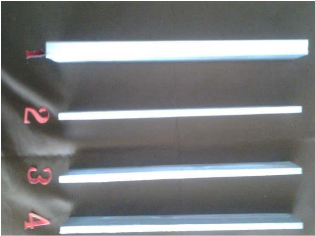
Picture# 4- After 18 hours in solution plates: # 2#3#4 were Reduced to (7.9 1x 0.79 x 0.03 inches)
