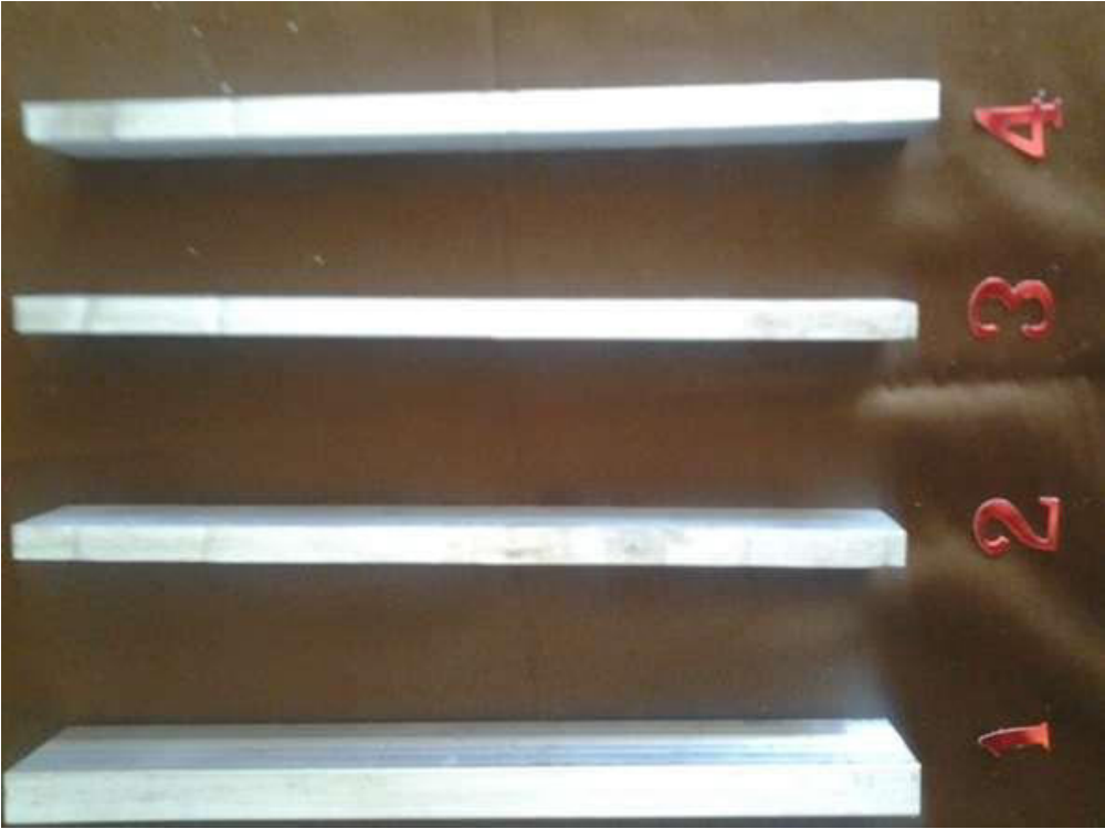
Picture #2- After 6 hours of stay in solution plates: # 2#3#4 were reduced to (8.71 x 1.1 x 0.41inches)
