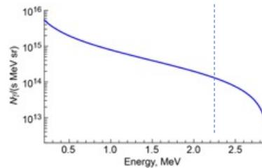
Produces gammas up to 2.9 MeV. At 0.45 mA per sample,  $\sim 2.9 \times 10^{12}$  gammas per s per sr. Photo-neutrons  $D(\gamma, n)p$  produced above 2.25 MeV, at  $E_n = 0.145$  MeV
