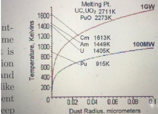
Figure 5. Equilibrium fuel particle temperature as a function of particle size.
