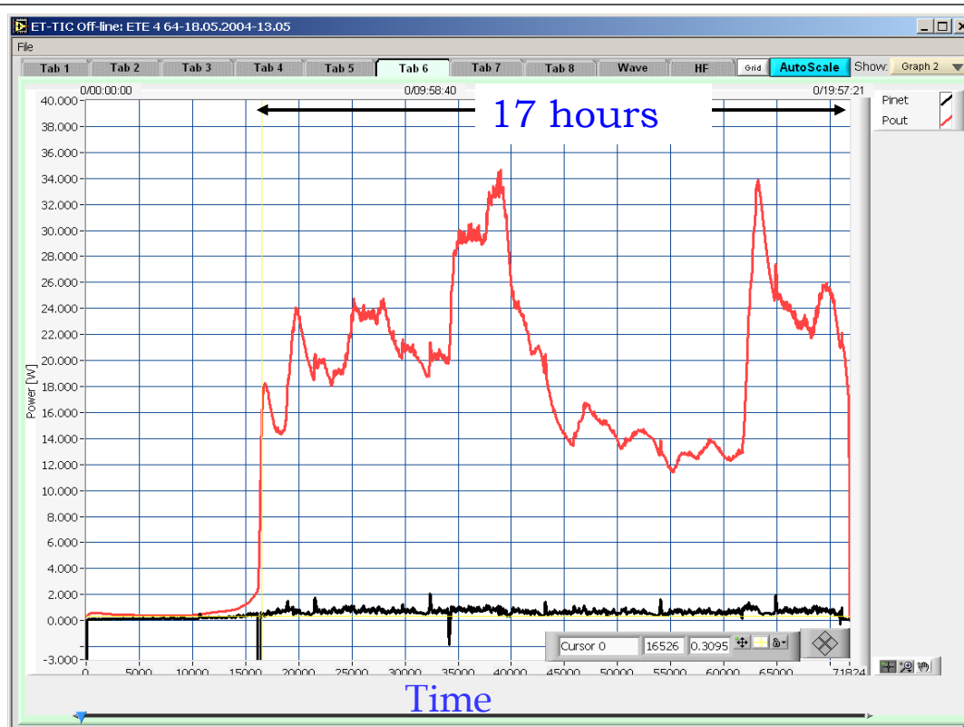
Figure 8. History of the electrical power into (black line) and thermal power out of (red line) an experiment by Energetics Technologies, which produced major LENR power for most on one day.
