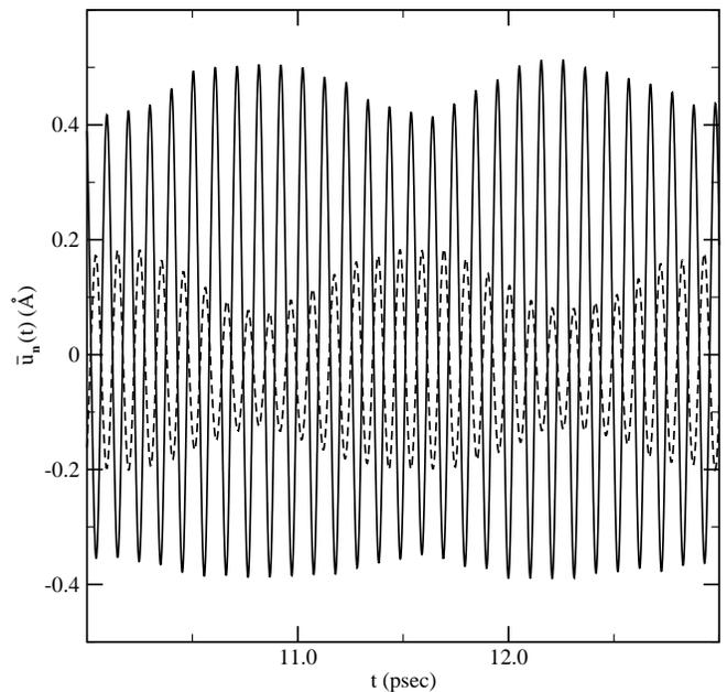
FIG. 3: Time dependence  $\bar{u}_n(t) = r_n(t) - r_0$  of the vibration of the central ( $n=0$ , solid line) and third ( $n=3$ , dashed line) bonds in Ni at long times containing the ILM with the frequency  $6.07 \cdot 10^{13}$  rad/sec. The corresponding values of the dc distortion  $\bar{\xi}_n$  are given in Table I. The amplitude modulation of the ILM is induced by its partner, the nearby linear local mode.
