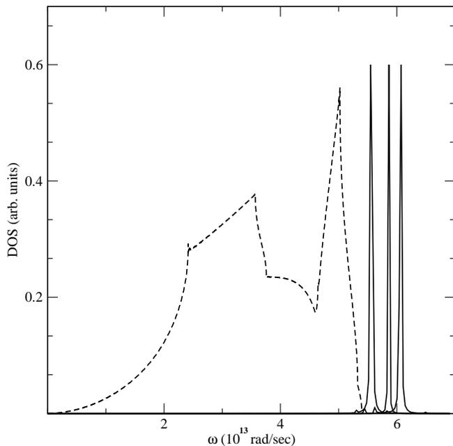
FIG. 2: Phonon density of states and three ILM spectral signatures for Ni. Phonon spectrum (dashed line) and spectrographs (solid line) of the different ILMs: The frequencies are 5.58, 5.86, 6.07 ( $10^{13}$  rad/sec) and the amplitudes of vibrations of the central bond are 0.18 Å, 0.31 Å and 0.42 Å.
