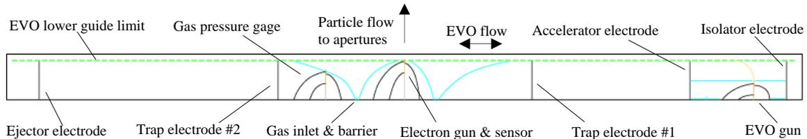
This ceramic structure, approximately 5 inches long, has a pattern of resistive materials on one surface that produce an EVO source, an electron gun for charging an EVO and producing a scatter spectrometer, an electron multiplier for analysis of EVO diameter, a gas pressure gage and various electrodes for trapping and acceleration. Two of these plates, one of them blank, are jointed together with a 0.002 inch space between them. Fig. 2 and Fig. 3 below show front and back views of the EVO guide.
