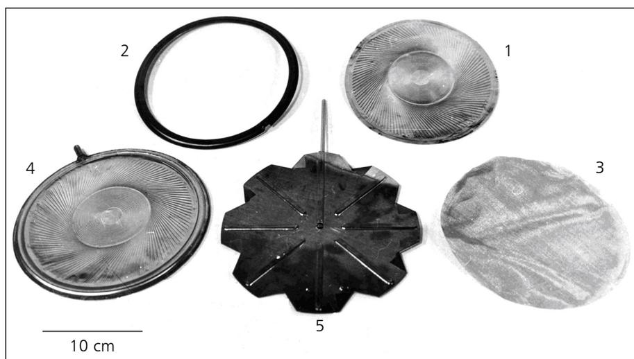
Fig. 2. Hydrogen separation element, its components, and gas distribution unit (deflector): 1 = palladium alloy membrane, 150 mm in diameter; 2 = ring frame; 3 = porous separator (wire netting); 4 = ready-assembled element; and 5 = deflector
