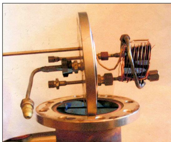
Fig. 4. Typical design of a membrane module with a hydrogen separation unit consisting of seven membrane elements with membranes 50 mm in diameter
