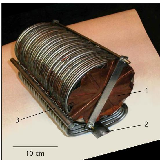
Fig. 3. Appearance of a hydrogen separation unit for the diffusion purification of hydrogen consisting of 50 diffusion elements with palladium-based alloy membrane 150 mm in diameter: 1 = deflector; 2 = high purity hydrogen outfall collector; and 3 = depleted mixture outfall collector
