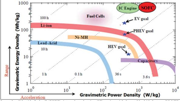
Legend: solid oxide fuel cell (SOFC); internal combustion (IC) engine; nickel-metal hydride battery (Ni-MH); hybrid-electric vehicles (HEV); electric vehicles (EV); and plug-in hybrid-electric vehicles (PHEV).
