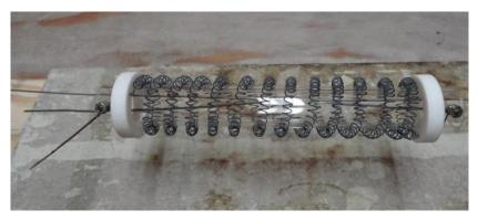
Figure 1: Oxidized Ni Wire Wound Around Quartz Tube
